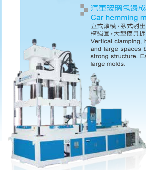
■ 四站圓盤雙機雙射 Four station disc dual machine injection 兩獨立射出系統，搭配轉盤，可做雙物件產品的一體成型。 Two independent injection systems with turntable to allow double injection.
